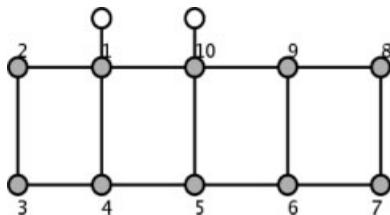
**Figure 3.** Coupling topology adapted to 10-8 symmetric characteristics.
