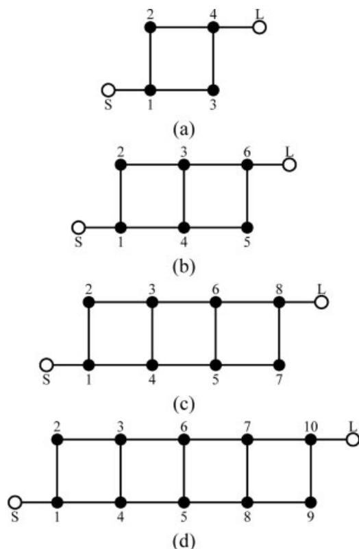
**Figure 1.** Coupling and routing diagrams for extended box section networks: (a) 4th degree (basic box section), (b) 6th degree, (c) 8th degree, and (d) 10th degree.
